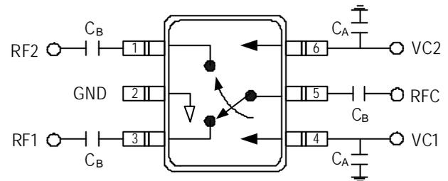
DC blocking capacitors  $C_B$  are required on all RF ports.
